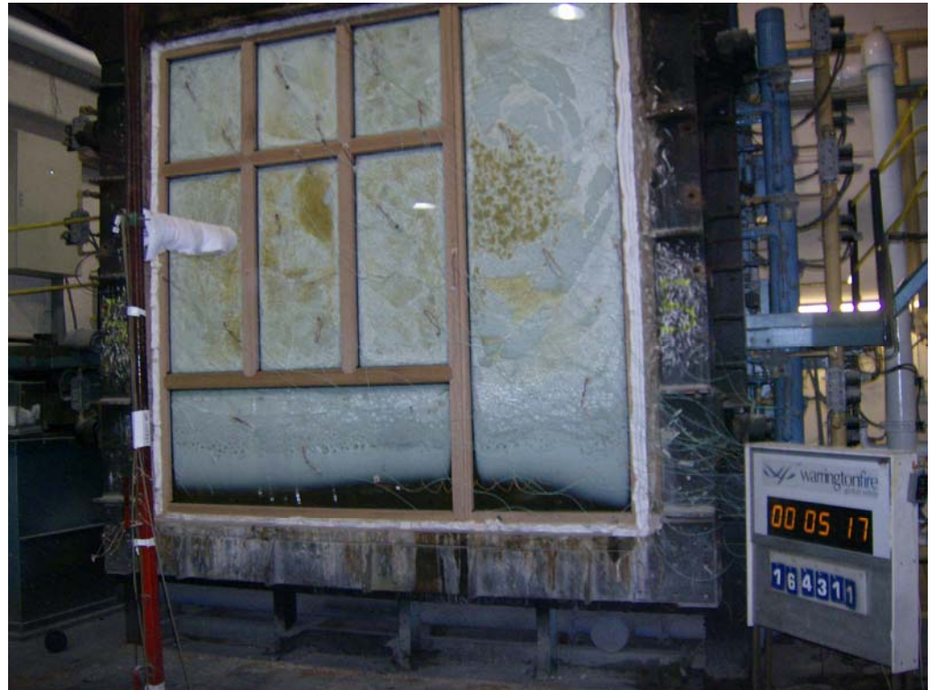
The unexposed face of the test construction after a test duration of 5 minutes
